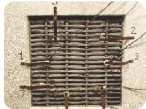
RCF grille after 60 minutes of fire resistance test (unexposed face)
