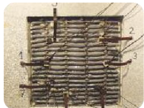
RCF grille after 30 minutes of fire resistance test (unexposed face)
