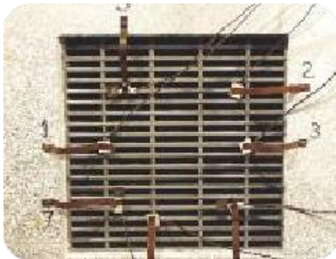
RCF grille after 30 minutes of fire resistance test (unexposed face)
