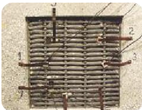
RCF grille after 30 minutes of fire resistance test (unexposed face)
