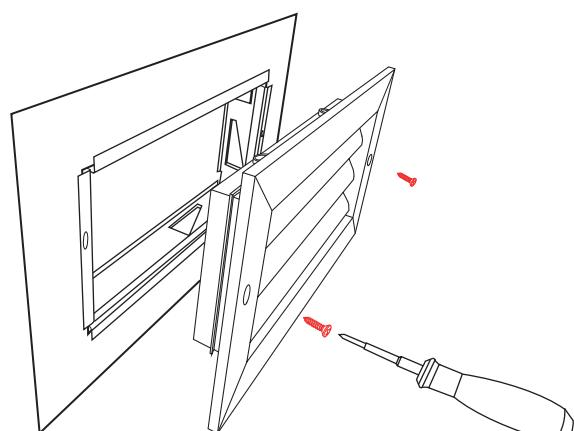
6 – Install the grille and fasten it using the screws and a screwdriver.
