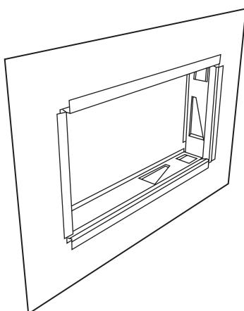
3 – Press the frame against the wall until it is positioned as shown in the image, and secure it by bending the latches.
