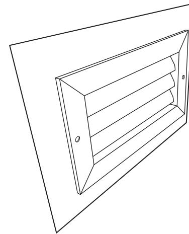
4 – Place the grille on top to mark the holes to be drilled.
