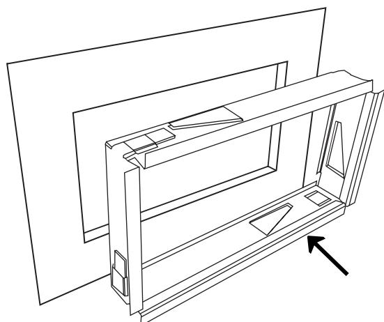
2 – Insert the mounting frame into the hole, pressing it firmly against the wall.
