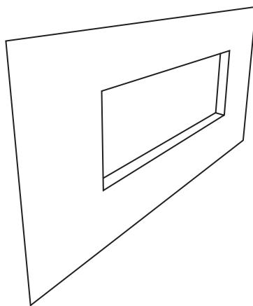
1 – Make a hole of the corresponding dimensions (check hole size in the catalogue) in the wall.
